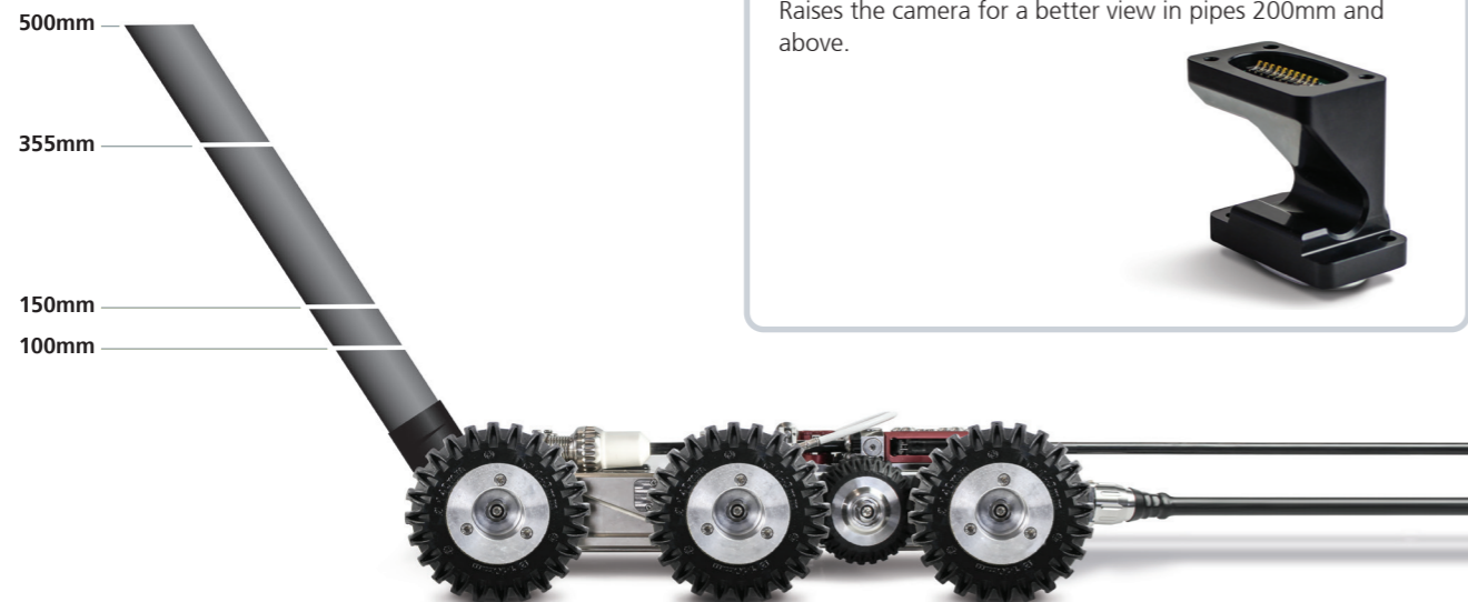
LAT150 with 140mm Soft Rubber Wheels (QRW140SR150)
