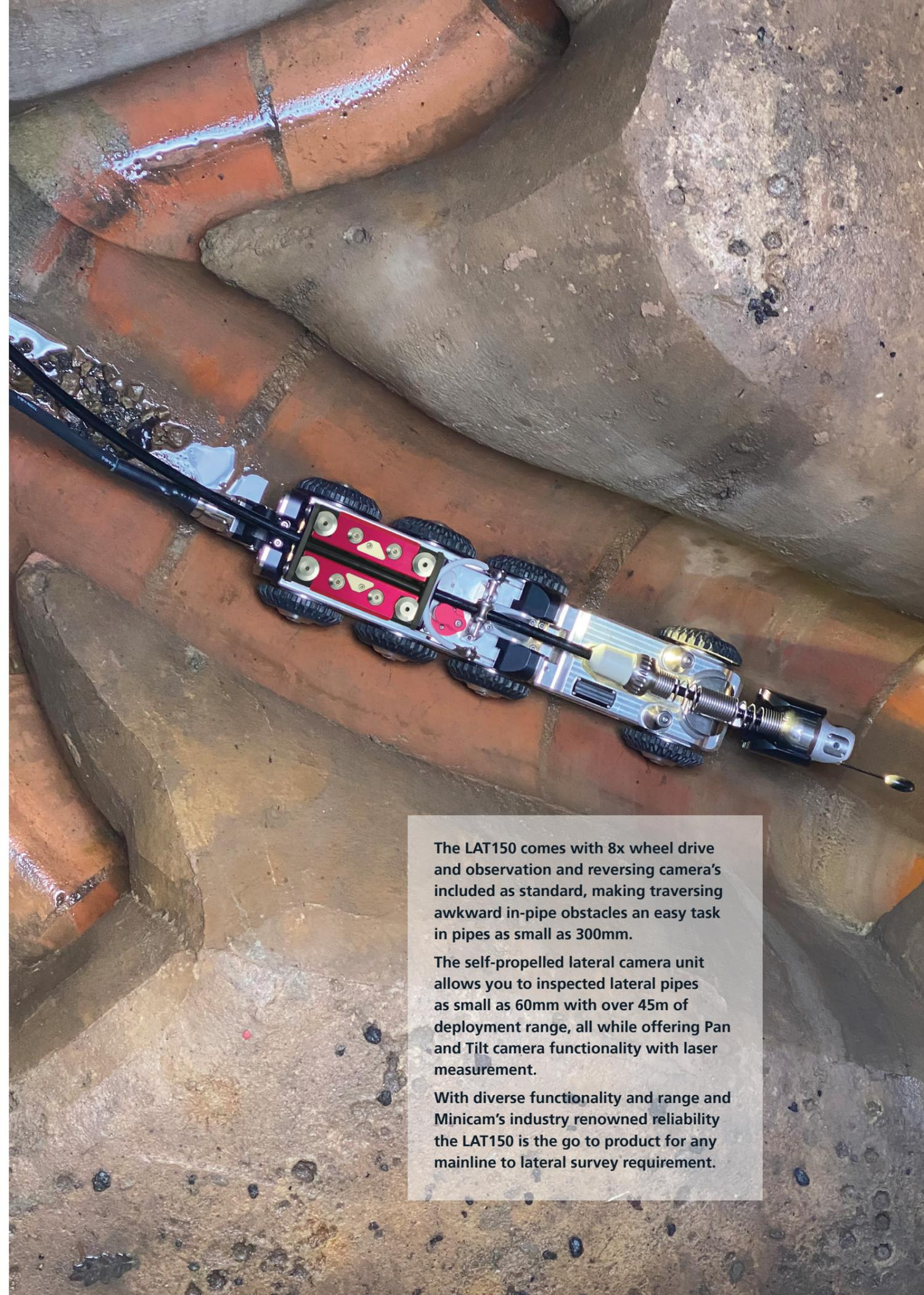
The LAT150 comes with 8x wheel drive and observation and reversing camera's included as standard, making traversing awkward in-pipe obstacles an easy task in pipes as small as 300mm.
