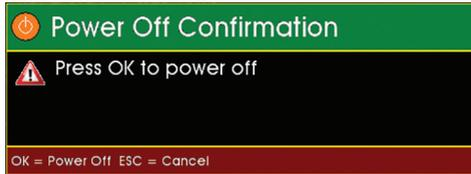
Press OK or the Carriage Return key and the unit will switch off in a controlled fashion.
