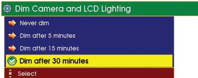
The camera illumination and LCD backlight will dim after a period of inactivity.
