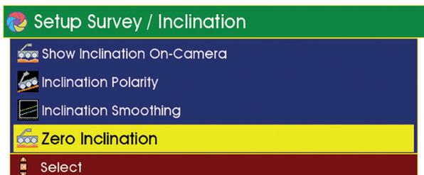
Select “Zero Inclination” and the first stage of the zero calibration begins:
