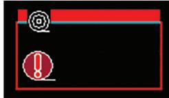
You can't control the cable reel or the crawler until the stop condition has been cleared.
