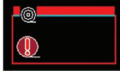
You can't control the cable reel or the crawler until the blockage condition has been cleared and reset.
