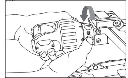
4 Turn the Locking Ring anti-clockwise as shown, to secure the camera in place.
