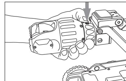
5 The position of the Locking Grub Screw should now be at the top (12 o'clock).
