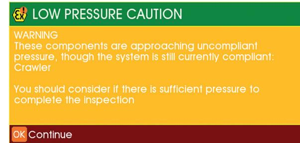
You must press OK to acknowledge this warning. The inspection equipment can still be used as the pressure is still Compliant.
