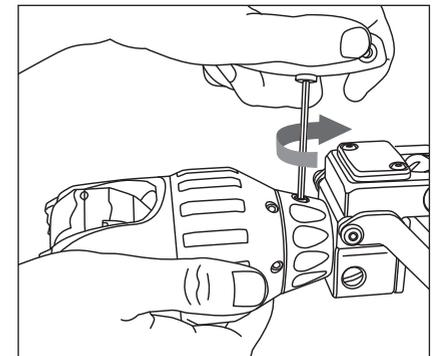
4 Use a 3mm T-Bar to screw and tighten the Locking Grub Screw. **DO NOT** over-tighten the Locking Grub Screw.
