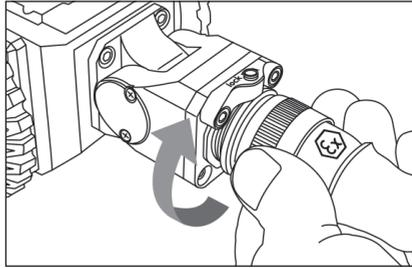
**2** Tighten the cable connector by turning in a clockwise direction as shown.
