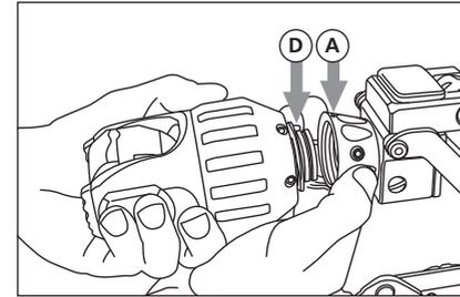
3 Offer the camera rear connector to the camera connector on the crawler, aligning the Orientation Pin (D) on the camera with the Orientation Dot (A) on the crawler.
