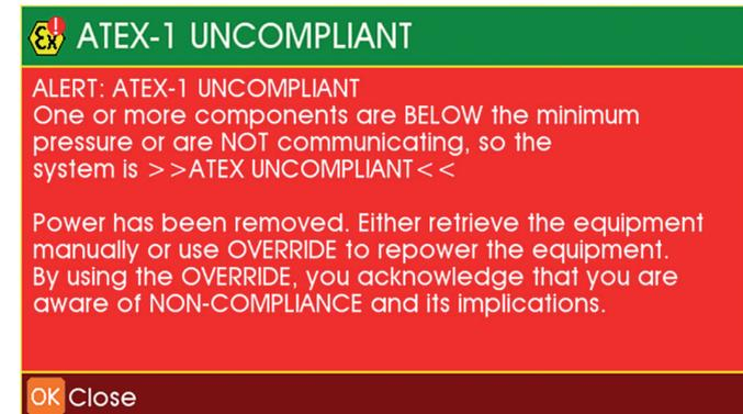
Press OK to acknowledge the alert, and then choose whether to continue using the Uncompliant inspection equipment by switching to OVERRIDE and powering ON again, or whether to abandon the survey and remove the
