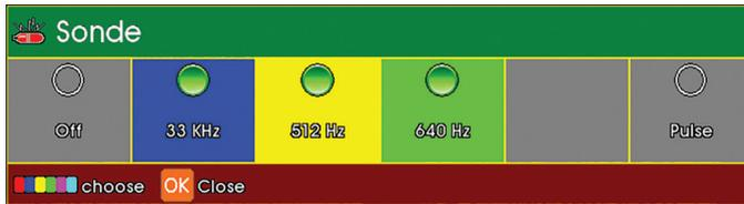
The Sonde can be cycled through three states – OFF, PULSED, ON.
