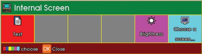
Press F6 (Cyan key) Choose a Screen to select the Internal Screen (CCU) or an External Monitor
