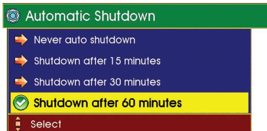
When the SOLOPro+ is powered only by internal batteries this feature will power down the SOLOPro+ after a period of inactivity.
