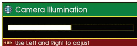
The Camera Illumination status bar will be displayed. Use the cursor control Left Arrow key to decrease the illumination. Use the cursor control Right Arrow key to increase the illumination.
